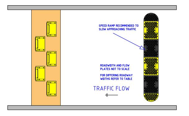
TRAFFIC FLOW CONTROL PLATES ARE DESIGNED TO ENCOURAGE ONE WAY TRAFFIC FLOW AND PREVENT UNAUTHORISED ENTRY/EXIT WITHIN ANY LOCATION.
